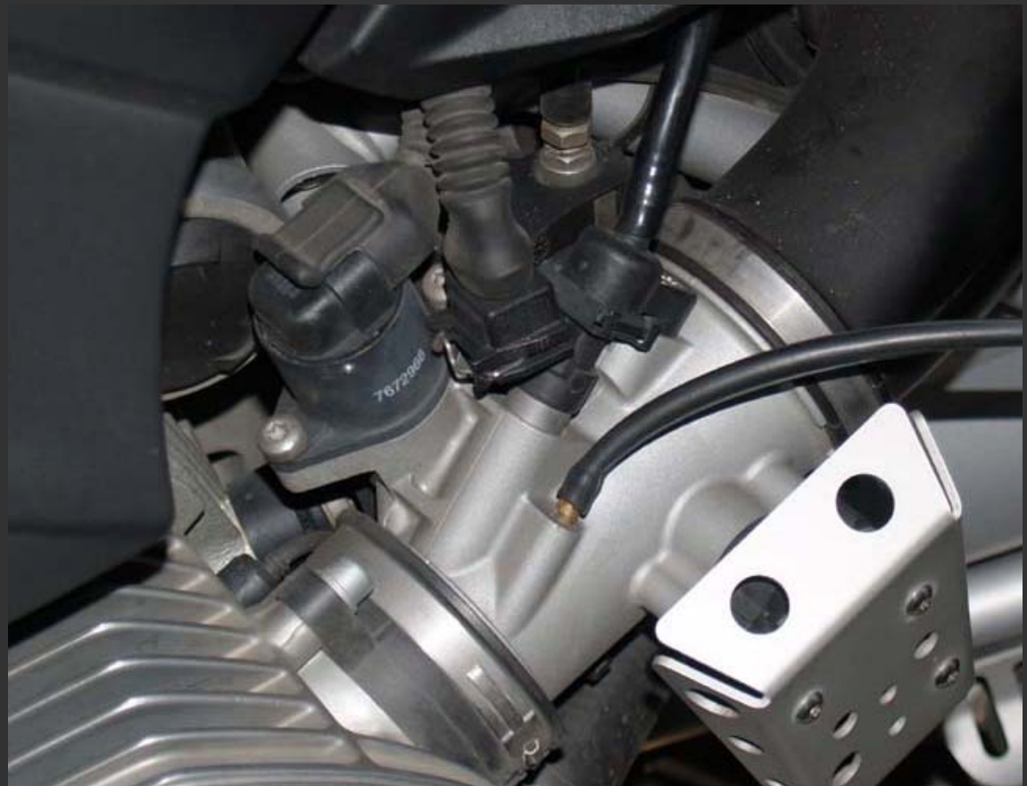
Here is a photo of the Twinmax hose installed.
