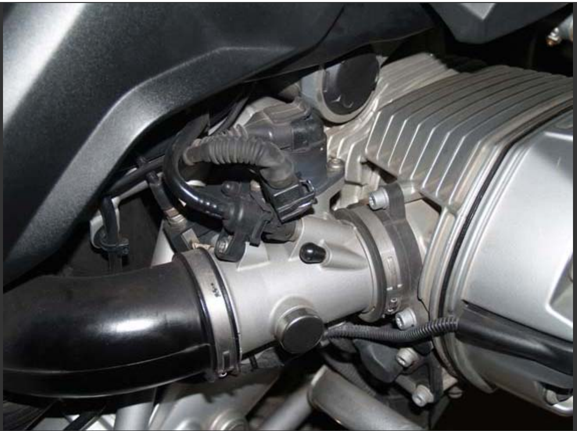
Here is the right side, and you put the other hose from the Twinmax here where the rubber cap is.
