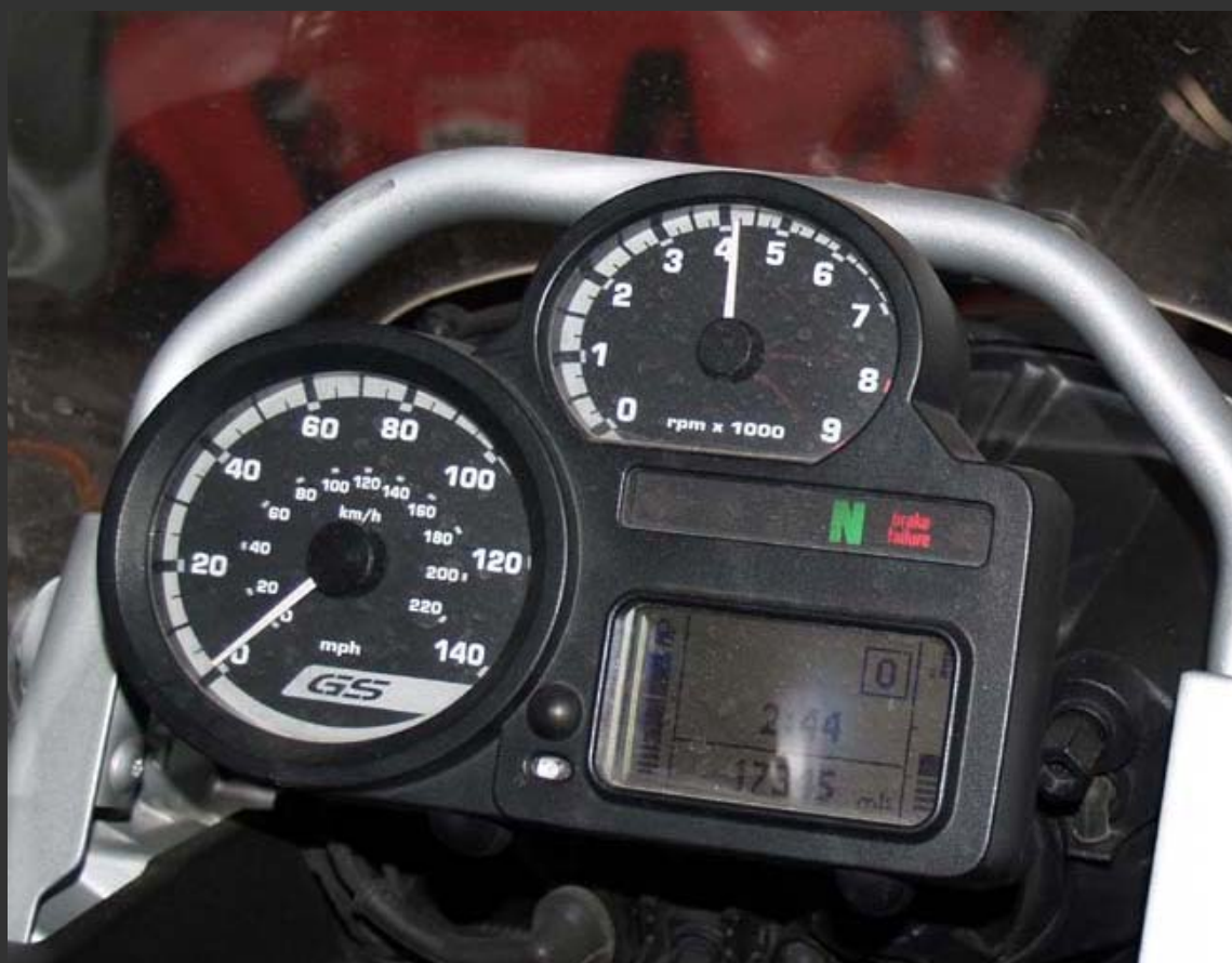
I then take it up to 3.5K RPM and check it again. (Note: I found that it is better to set the cable sync at about 3000-3500.)
